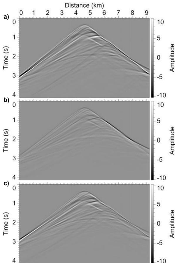
**Figure 4.** The (a) observed data computed using the true background slowness shown in Figure 2 and true reflectivity shown in Figure 3a for a source located at distance 4.6 km, (b) simulated data computed using the true background slowness scaled by 95% and reflectivity shown in Figure 3c, and (c) simulated data computed using the true background slowness scaled by 95% and reflectivity shown in Figure 3d. Note the similarity in amplitude between the observed data (a) and simulated data (c).
