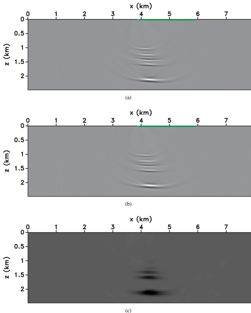
**Figure 9.** (a) Baseline image, (b) monitor image obtained using the baseline velocity model, (c) relative shifts between the two images. Black indicates positive (downward) shifts and white represents negative (upward) shifts. Here, the migration velocity model is 5% faster than the correct one.
