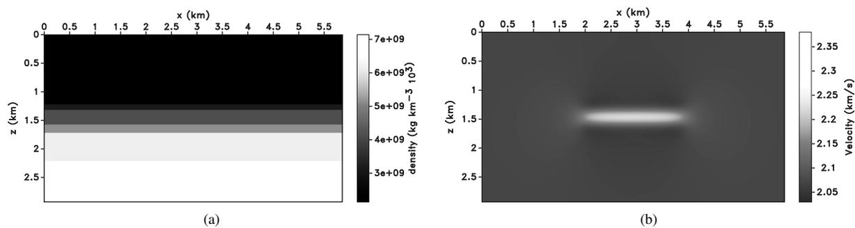
**Figure 11.** (a) Density model used to simulate the reflecting interfaces. (b) Velocity model of the depleted reservoir. The original model is homogeneous with 2.07 km/s velocity. Observe the characteristic shape of the anomaly with increasing velocity inside the reservoir (because of compaction) and decreasing velocity outside the reservoir (because of strain).
