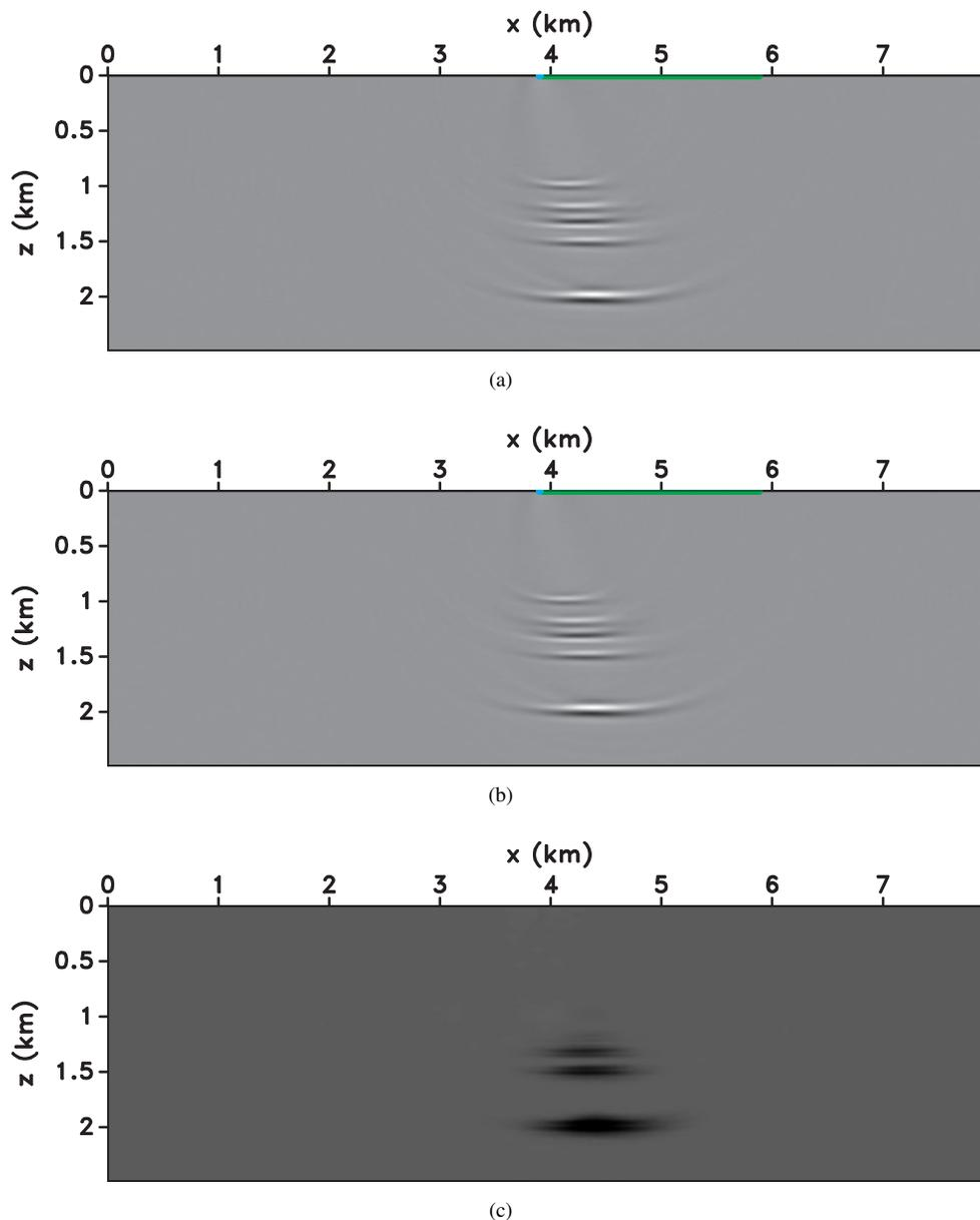
**Figure 7.** (a) Baseline image, (b) monitor image obtained using the baseline velocity model, and (c) relative shifts between the two images. Black indicates positive (downward) shifts and white represents negative (upward) shifts. The baseline migration model is kinematically accurate and the error is due only to 4D effects in the monitor survey.
