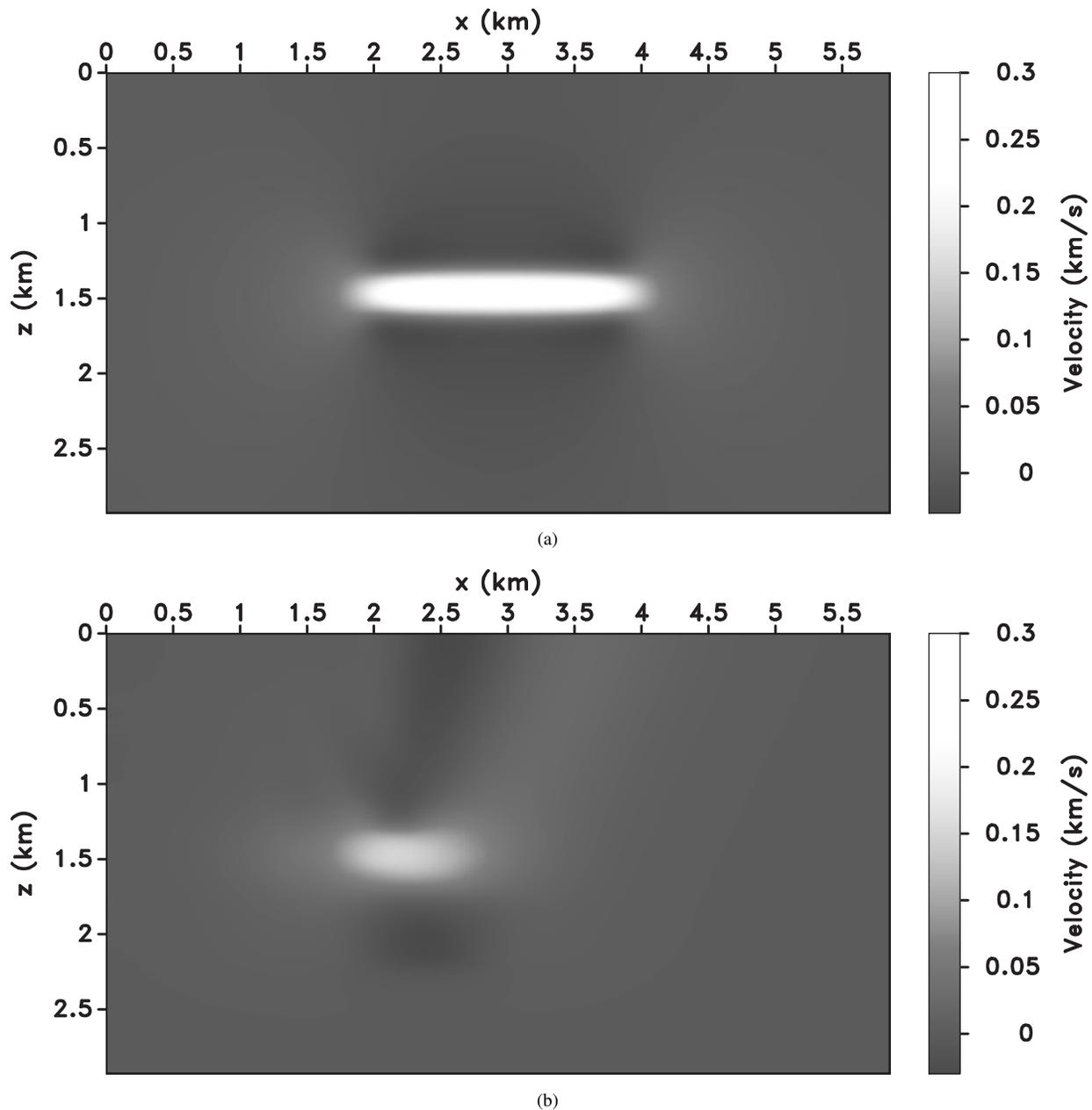
**Figure 13.** (a) Real time-lapse model perturbation and (b) inverted perturbation after 60 iterations of wavefield tomography. Notice that we are able to correctly image the anomaly and also constrain its lateral extent at about  $x = 2$  km.
