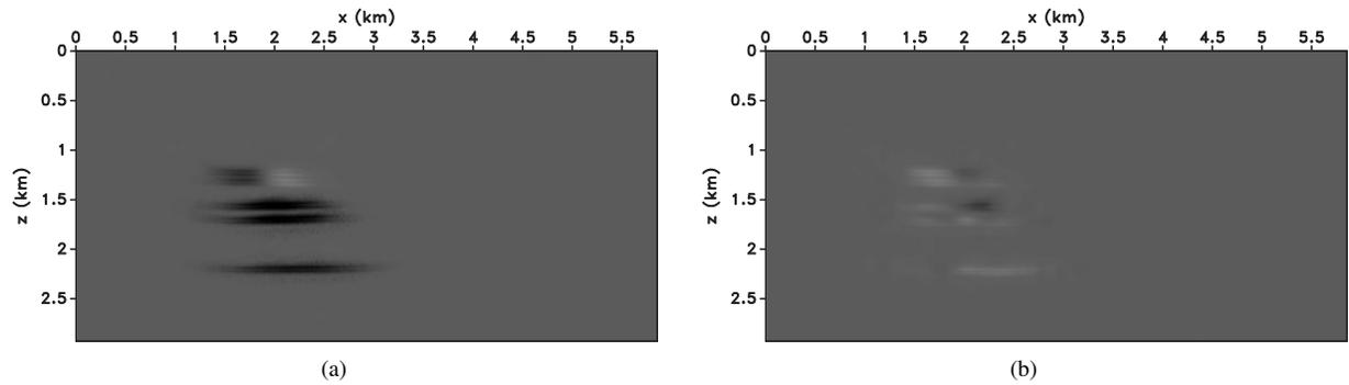
**Figure 14.** (a) Initial estimated shifts and (b) estimated shifts after 60 iterations of wavefield tomography. Black indicates positive (downward) shifts and white represents negative (upward) shifts. Inversion matches the baseline and monitor images and reduces the shifts between them.
