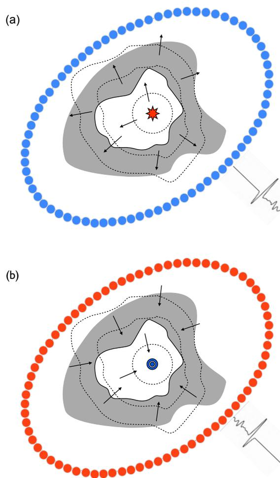
**Figure 1.** Illustration of a time-reversal experiment. (a) Forward propagation step: waves excited by a source travel through the complex medium and are recorded at stations marked as circles. (b) Back-propagation step: the recorded signals are reversed in time and re-emitted into the medium at the corresponding stations. The waves then propagate through the medium and converge on the original source location. Figure from (Lu, 2002).
