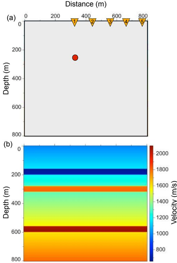
**Figure 2.** Configuration of the synthetic experiment (a) showing the locations of the sources (yellow triangles) and focusing target (red circle), and the assumed acoustic velocity model (b) for the medium.
