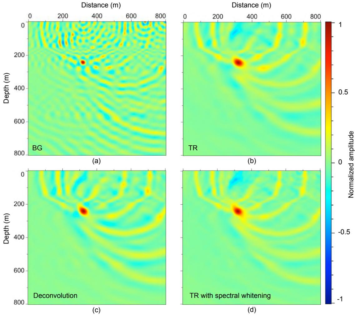
**Figure 6.** Same results as in Figure 5 for the same data plus bandlimited noise to simulate a microseismic location experiment. The plots show the snapshots of propagating wavefields at the time of focus for (a) BG (the proposed method), (b) time-reversal, (c) deconvolution, and (d) time-reversal with spectral whitening.
