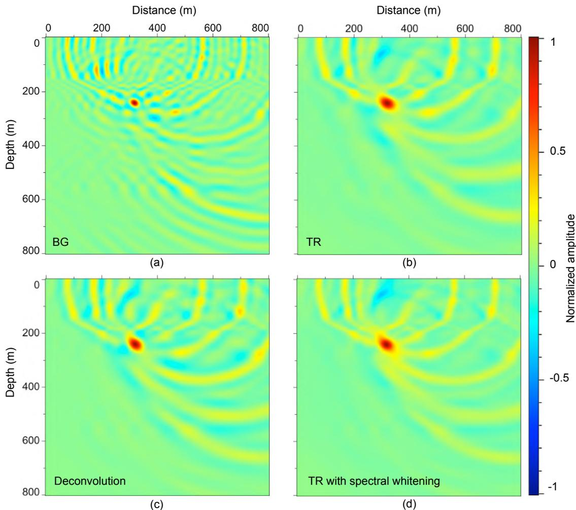
**Figure 5.** Results of the numerical focusing experiment of section 4 using noise-free data. The plots show the snapshots of propagating wavefields at the time of focus for (a) BG (the proposed method), (b) time-reversal, (c) deconvolution, and (d) time-reversal with spectral whitening.
