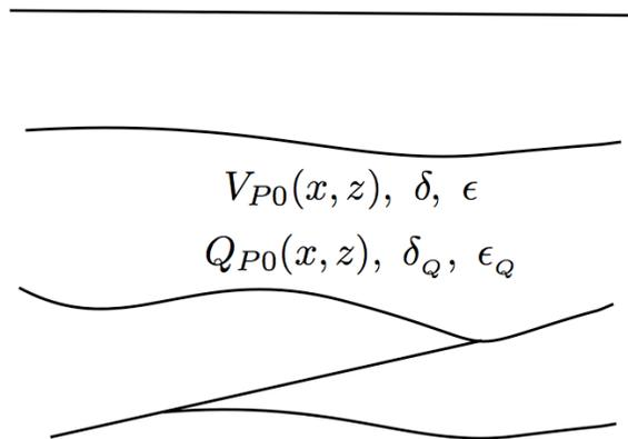
**Figure 3.** 2D model for velocity and attenuation estimation. The subsurface is divided into factorized blocks with VTI symmetry for both velocity and attenuation. The P-wave vertical velocity and quality factor are assumed to vary linearly with depth and lateral position, while the velocity-anisotropy parameters  $\epsilon$  and  $\delta$  and the attenuation-anisotropy parameters  $\epsilon_Q$  and  $\delta_Q$  within each block are constant.
