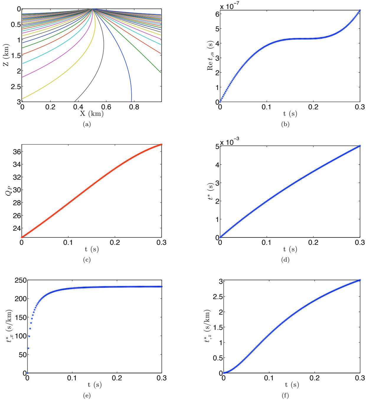
**Figure 2.** Ray-tracing results for model 3 from Table 1. (a) Ray trajectories. (b) Perturbation of the real-valued traveltime as a function of the unperturbed traveltime along the ray. (c) The quality factor  $Q_P$ , (d) dissipation factor  $t^*$ , and the spatial derivative of the dissipation factor with respect to (e)  $x$  and (f)  $z$  computed along the ray with a take-off phase angle of  $18^\circ$ .
