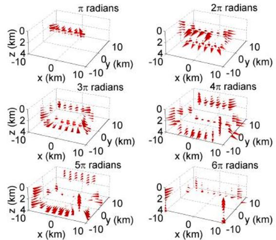
**Figure 14.** The phase-binned gradient of a scalar diffusive field with five synthetic aperture sources steered in the crossline direction at  $45^\circ$ . The energy is moving asymmetrically in the negative  $y$ -direction in contrast to the symmetric movement of the unsteered field.
