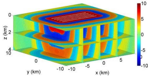
**Figure 3.** The unsteered 3D scalar diffusive field log-transformed.
