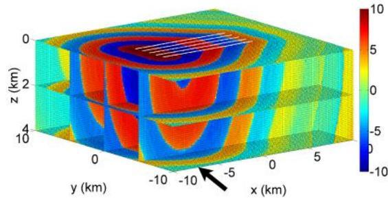
**Figure 4.** The 3D scalar diffusive field log-transformed and steered at a  $45^\circ$  angle in the inline direction. The arrow shows the shift in the x-direction of the energy from the origin; without steering the maximum energy would be located at the center of the source lines ( $x=0\text{km}$ ).
