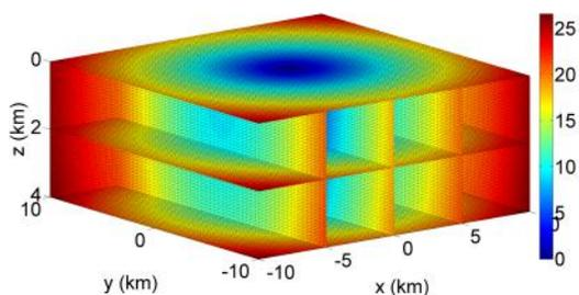
**Figure 7.** The unwrapped phase of a scalar diffusive field from a point-source located at (0,0,0). The colorbar displays radians.
