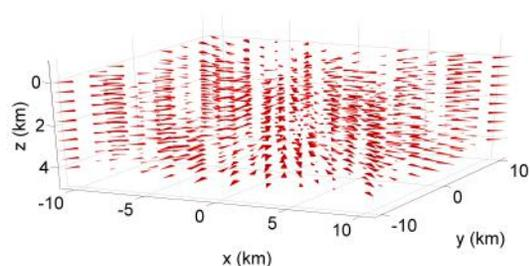
**Figure 8.** The normalized gradient of a scalar diffusive field from a point-source location at (0,0,0).
