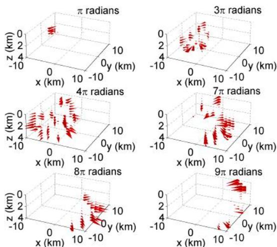
**Figure 15.** The phase-binned gradient of a scalar diffusive field steered in the inline and crossline directions at  $45^\circ$ . The combined inline and crossline steering produces a field whose energy moves out asymmetrically in both the  $x$ - and  $y$ -directions.
