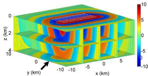
**Figure 5.** The 3D scalar diffusive field log-transformed and steered at a  $45^\circ$  angle in the crossline direction. The arrow shows the shift in the energy from the centerline of the survey ( $y=0\text{km}$ ). The shift is less than in Figure 4 because fewer sources are used.
