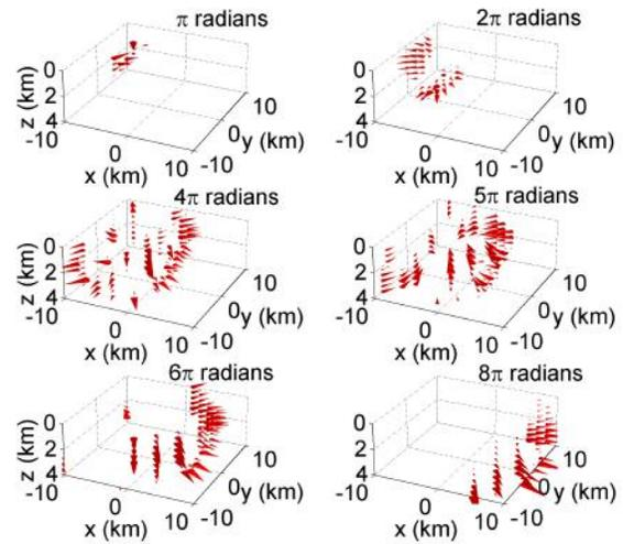
**Figure 13.** The phase-binned gradient of a scalar diffusive field with five synthetic aperture sources steered in the inline direction at a  $45^\circ$ . The energy is moving asymmetrically in the  $x$ -direction unlike the symmetric movement of the unsteered field.
