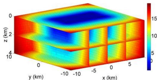
**Figure 10.** The unwrapped phase of a scalar diffusive field with five lines of synthetic aperture sources. The colorbar displays radians.
