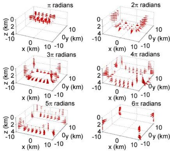
**Figure 12.** The phase-binned gradient of a scalar diffusive field with five unsteered synthetic aperture sources. The movement of the energy is symmetric about both the  $x$  and  $y$  directions.
