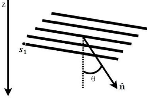
**Figure 1.** The design of a traditional CSEM survey. The individual source,  $\mathbf{s}_1$ , is defined to be located at the origin. The steering angle,  $\hat{\mathbf{n}}$ , is a function of  $\theta$ , the dip and  $\varphi$  which is either  $0^\circ$  or  $90^\circ$  to steer in the inline or crossline directions, respectively.
