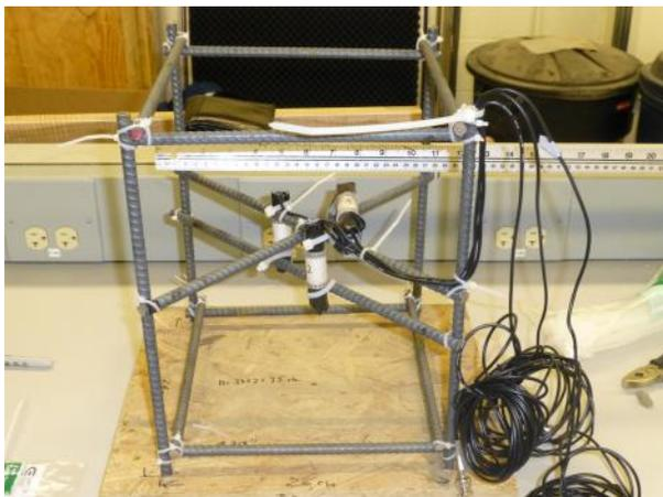
Source set up and reinforcement placed within the concrete block
