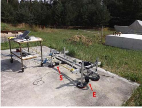
**Figure 11.** Scanner on the foundation slab with transmitting (S) and receiving (E) ultrasonic transducer arrays
