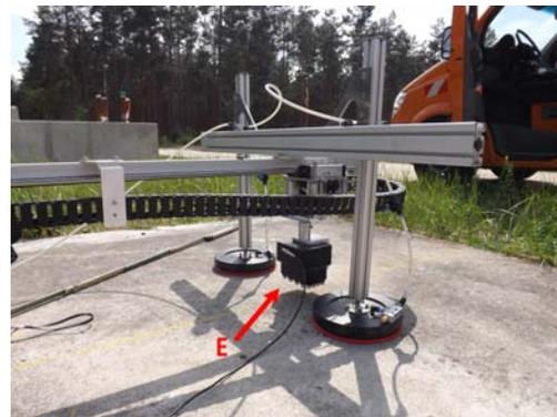
Figure 10. Scanner on the foundation slab moving the receiving transducer array (E)
