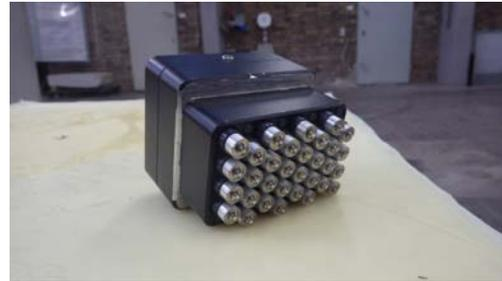
Figure 9. Ultrasonic transducer array consisting of 32 dry point contact transducers
