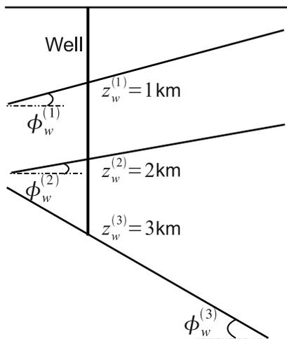
**Figure 5.** Three-layer TTI model used to test the tomographic algorithm. The dips are  $\phi_w^{(1)} = 15^\circ$ ,  $\phi_w^{(2)} = 10^\circ$ , and  $\phi_w^{(3)} = -30^\circ$ . The reflector depths at the well location are  $z_w^{(1)} = 1$  km,  $z_w^{(2)} = 2$  km, and  $z_w^{(3)} = 3$  km.
