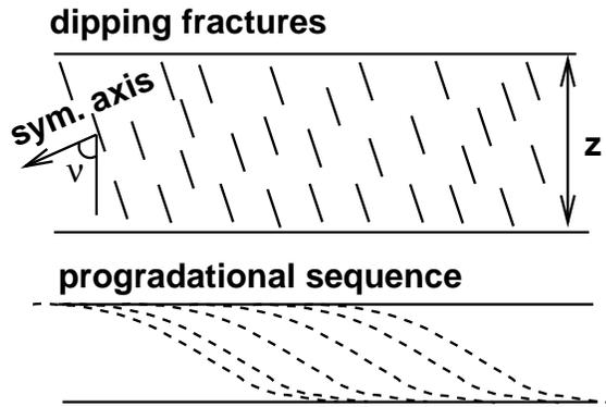
**Figure 1.** TI layer with a tilted symmetry axis describes progradational sequences and a system of obliquely dipping, penny-shaped fractures embedded in isotropic host rock (after Dewangan & Tsvankin, 2006a).
