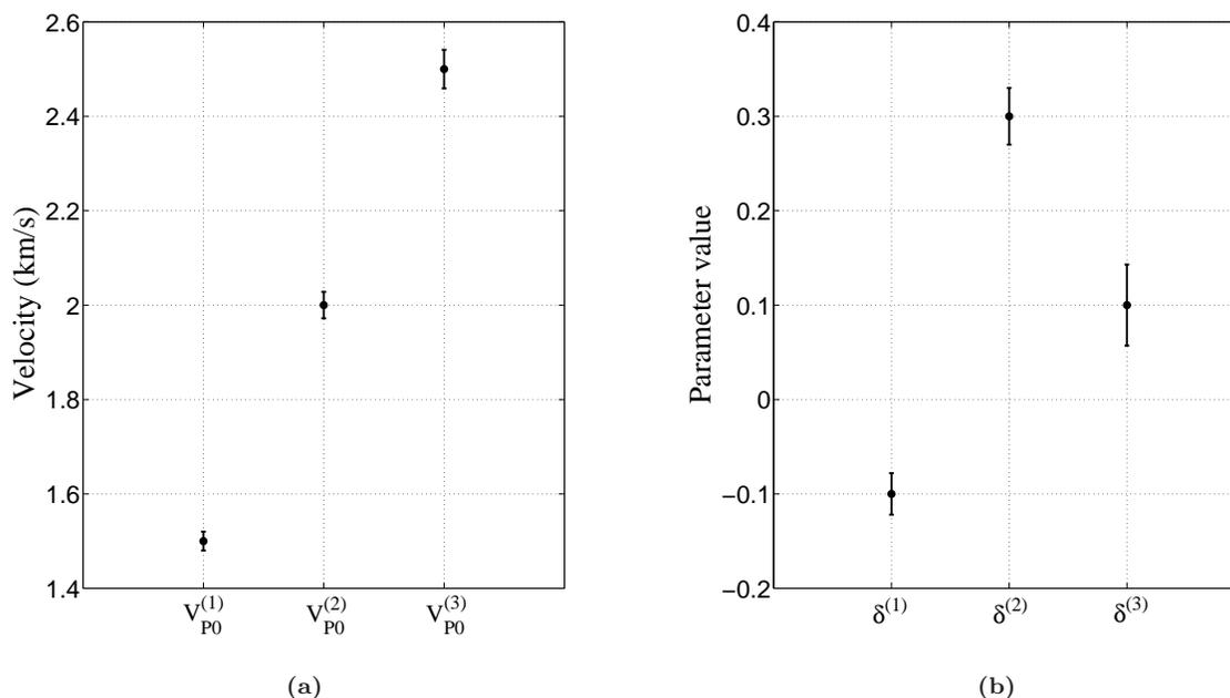
**Figure 6.** a) Interval symmetry-direction velocities  $V_{P0}^{(n)}$  and b) anisotropy parameters  $\delta^{(n)}$  ( $n = 1, 2, 3$ ) estimated by the tomographic inversion for the model from Figure 5 and Table 4. The dots mark the exact values, and the bars correspond to the  $\pm$  standard deviation in each parameter.
