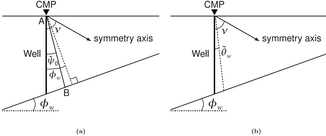
**Figure 3.** Dipping TTI layer with the CMP at the head of a vertical well. The arrow marks the symmetry axis; the reflector dip is  $\phi_w$ . a) AB is the zero-offset raypath; the group and phase angles of the zero-offset ray with the vertical are  $\tilde{\psi}_0$  and  $\phi_w$ , respectively. b) The phase-velocity vector of the vertical ray makes the angle  $\tilde{\theta}_w$  with the vertical.
