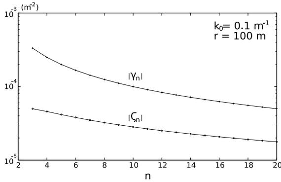
**Figure 5.** Comparison of the absolute values of  $\gamma_n$  and  $\zeta_n$  in equation (33). For  $k_0 = 0.1 \text{ m}^{-1}$  and  $r = 100 \text{ m}$ ,  $|\zeta_n|$  is much smaller than  $|\gamma_n|$ . The two terms are dependent on  $k_0/r$  and  $1/r^2$ , respectively, which implies  $\gamma_n$  is significant at a large source-receiver offset and for a large wavenumber of the reference medium.
