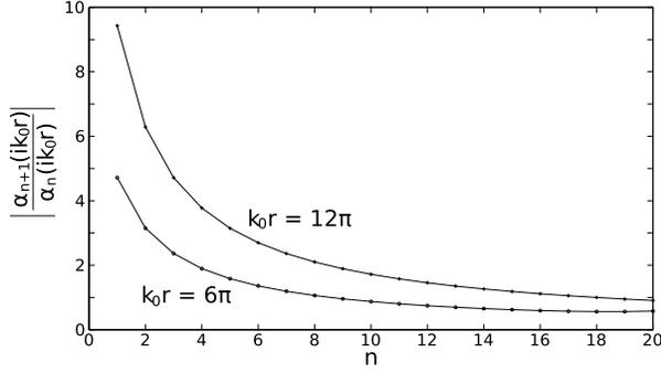
**Figure 4.** Convergence rate of forward scattering series. The ratio  $|\alpha_{n+1}/\alpha_n|$  in equation (30) for increasing number of  $n$  is compared at two spatial locations: one is 3 wavelengths apart from the source ( $k_0 r = 6\pi$ ) and the other is 6 wavelengths ( $k_0 r = 12\pi$ ).
