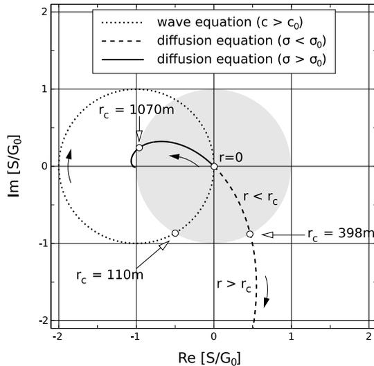
**Figure 12.** The variation of  $S/G_0$  in the complex plane for different values of  $r$ . The origin of the complex plane indicate  $r = 0$ , and the arrows denote the directions of increasing  $r$ . Three different cases shown in Figures 8, 9, and 11 are compared. The shaded region denotes the area where the inverse series converges.
