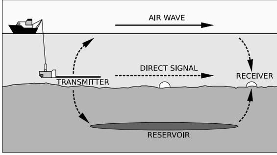
**Figure 3.** Schematic representation of controlled-source electromagnetic (CSEM) exploration from MacGregor et al. (2006). An electromagnetic transmitter is towed close to the seafloor to maximize the coupling of electric and magnetic fields with seafloor rocks. These fields are recorded by receivers deployed on the seafloor some distance from the transmitter.
