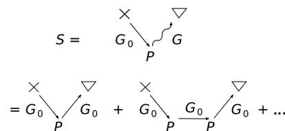
**Figure 2.** Schematic illustration of the forward scattering series from Weglein et al. (2003). The symbols  $\times$  and  $\nabla$  indicate source and receiver.  $S$ ,  $P$ ,  $G_0$ , and  $G$  are the scattered field, perturbation, and Green functions for the reference and actual media, respectively. The straight and wiggled arrows indicate signals through the reference and perturbed media, respectively.
