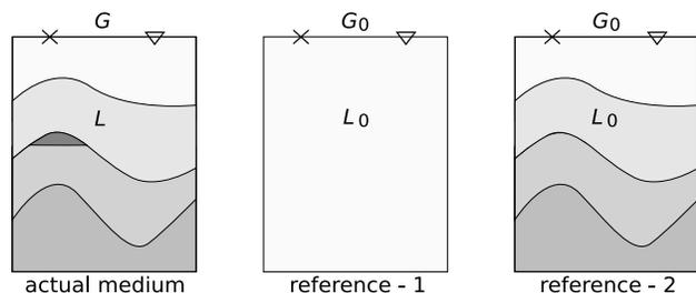
**Figure 1.** Actual medium versus different choices of reference medium. The symbols  $\times$  and  $\nabla$  indicate the source and receiver, respectively.  $G$  and  $G_0$  are the Green functions for the actual and reference media, respectively. Note that given the actual medium, there are several possible choices of the reference medium.
