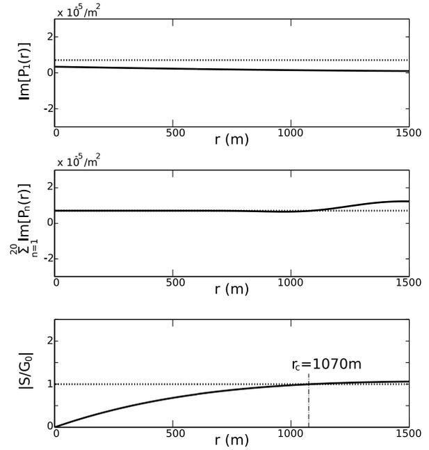
**Figure 11.** Spatial variation of the inverse scattering series for the electromagnetic diffusion equation (imaginary part only). The medium properties of the perturbed and reference media are switched from the previous case shown in Figure 9 and Table 1. Note that the spatial range where  $|S(\mathbf{r})/G_0(\mathbf{r})| < 1$  is wider than the case shown in Figure 9.
