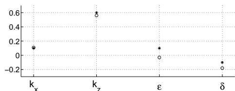
**Figure 18.** Estimated ( $\circ$ ) and true ( $\star$ ) parameters of the second layer obtained with an inaccurate value of the vertical velocity at the top of the second layer [ $V_{P0}(x = 4000 \text{ m}, z = 800 \text{ m}) = 2600 \text{ m/s}$ ].
