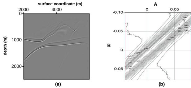
**Figure 2.** (a) Image of the model from Figure 1 obtained using a homogeneous isotropic velocity field with  $V_{P0} = 2600 \text{ m/s}$ . (b) Semblance contour plot computed from equation (5) for the shallow reflector at the surface location 3 km.
