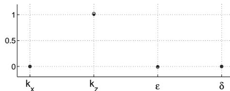
**Figure 14.** Estimated (o) and true (\*) parameters of the first layer obtained using the correct  $V_{P0}(x = 4000 \text{ m}, z = 0 \text{ m}) = 1500$  m/s on the surface.
