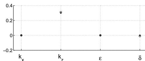
**Figure 19.** Estimated ( $\circ$ ) and the true ( $\star$ ) parameters of the third layer obtained with an inaccurate value of the vertical velocity at the top of the second layer [ $V_{P0}(x = 4000 \text{ m}, z = 800 \text{ m}) = 2600 \text{ m/s}$ ] but the correct  $V_{P0}(x = 4000 \text{ m}, z = 1208 \text{ m}) = 2732 \text{ m/s}$  at the top of the third layer.
