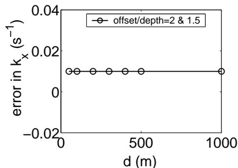
**Figure 9.** Influence of the distance between the two horizontal reflectors on the absolute error in the horizontal gradient  $k_x$ . The parameters are the same as in Figure 8.
