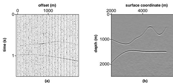
**Figure 6.** Influence of noise on the velocity analysis and migration. (a) A shot gather from the dataset in Figure 1 after the addition of Gaussian noise; the signal-to-noise ratio is 1.5. (b) The image obtained for the noisy dataset.
