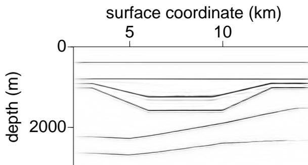
**Figure 20.** Stacked image obtained after prestack depth migration using the estimated parameters from Figures 14, 18, and 19. The vertical velocity  $V_{P0}$  at the top of the second layer was inaccurate.
