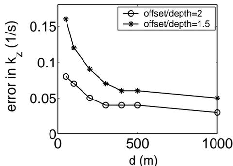
**Figure 8.** Influence of the vertical distance  $d$  between the two horizontal reflectors used in the velocity analysis on the absolute error in the vertical gradient  $k_z$ . The depth of the shallow reflector is 1 km; the maximum offset is 2 km for the upper curve and 1.5 km for the lower curve. The model parameters are  $V_{P0}(x = 3 \text{ km}, z = 0) = 2600 \text{ m/s}$ ,  $k_z = 0.6 \text{ s}^{-1}$ ,  $k_x = 0.2 \text{ s}^{-1}$ ,  $\epsilon = 0.2$ , and  $\delta = 0.1$ .
