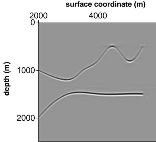
**Figure 1.** True image of two reflectors embedded in a factorized  $v(x, z)$  VTI medium with the parameters  $V_{P0}(x = 3 \text{ km}, z = 0) = 2600 \text{ m/s}$ ,  $k_z = 0.6 \text{ s}^{-1}$ ,  $k_x = 0.2 \text{ s}^{-1}$ ,  $\epsilon = 0.1$ , and  $\delta = -0.1$ . The corresponding effective parameters are  $V_{\text{nmo}}(x = 3 \text{ km}, z = 0) = 2326 \text{ m/s}$ ,  $k_z = 0.6 \text{ s}^{-1}$ ,  $\hat{k}_x = 0.18 \text{ s}^{-1}$ , and  $\eta = 0.25$ .
