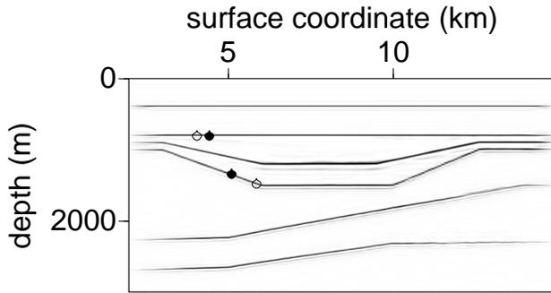
**Figure 23.** Stacked image obtained after prestack depth migration using the estimated parameters from Figures 14, 21, and 22. The vertical velocity was assumed to be continuous between the first and second layers at the point ( $x = 3900$  m,  $z = 800$  m) and between the second and third layers at the point ( $x = 5937$  m,  $z = 1483$  m). True (●) and estimated (○) points of continuity are also indicated.
