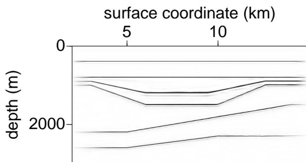
**Figure 17.** Stacked image obtained after prestack depth migration using the estimated parameters from Figures 14–16. The vertical velocity  $V_{P0}$  at the top of each layer was known.
