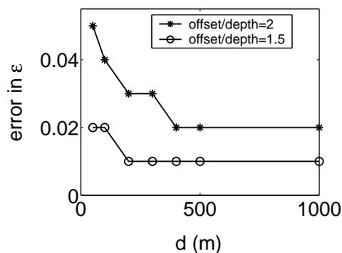
**Figure 10.** Influence of the distance between the two horizontal reflectors on the absolute error in the parameter  $\epsilon$ . The parameters are the same as in Figure 8.
