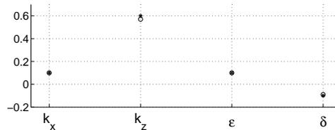
**Figure 15.** Estimated (o) and true (\*) parameters of the second layer obtained using the correct  $V_{P0}(x = 4000 \text{ m}, z = 800 \text{ m}) = 2300$  m/s at the layer's top.
