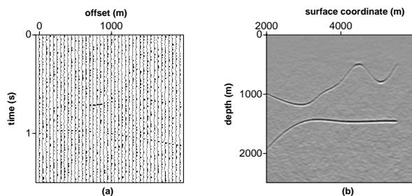
**Figure 7.** Influence of noise on the velocity analysis and migration. (a) The same shot gather as in Figure 6, but with a more severe noise contamination (signal-to-noise ratio is 1). (b) The image obtained for the noisy dataset.
