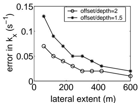
**Figure 12.** Influence of the lateral spread of the image gathers on the absolute error in  $k_x$ . The reflector depths are 1 km and 1.2 km; the other parameters are the same as in Figure 10. The velocity analysis is performed on 12 image gathers (each with 20 offsets).
