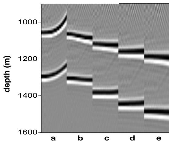
**Figure 4.** Residual moveout in image gathers for both reflectors at the surface location 3 km: (a) for the initial model; (b) after two, (c) four, (d) six, and (e) eight iterations. The residual moveout is minimized during the velocity-updating process.
