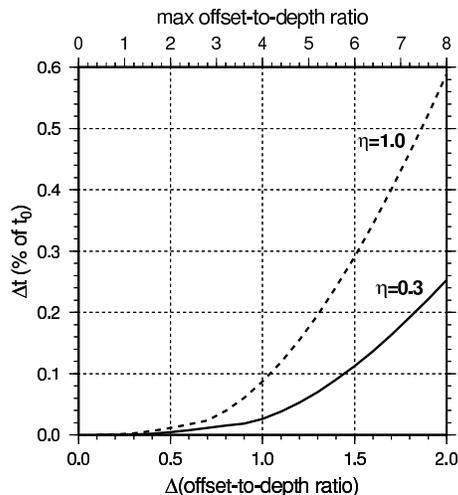
**Figure 5.** Accuracy of the  $[2/2]$  rational interpolation as a function of the separation in ODR of the interpolation traveltimes for  $\eta = 0.3$  and  $\eta = 1.0$ . In both cases  $V_{NMO} = 2.4$  km/s. Even if the separation in ODR is two, i.e., the maximum ODR is 8, the percentage errors in traveltime are of the order  $10^{-1}$ .
