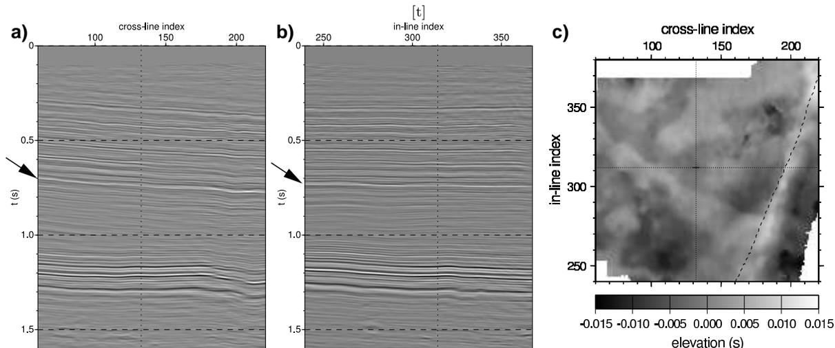
**Figure 9.** Field data used to test the rational interpolation method. Inline (a), crossline (b), and plan view of the residual topography of the event used for testing (indicated by the arrows in a and b) after removal of the regional dip (c). The dotted lines in c denote the locations of the inline and crossline sections shown in a and b. The dashed line in c denotes the location of a regional fault.
