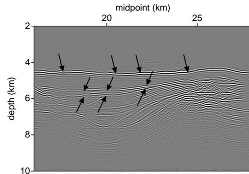
**Figure 20.** This figure repeats the estimated artifacts from internal multiples shown in Figure 19, with arrows indicating locations at which multiples can be observed in the results of ten Kroode (2005).
