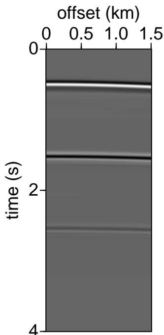
**Figure 3.** Top: Velocity model for flat example. Bottom: Surface data (CMP) for flat example.
