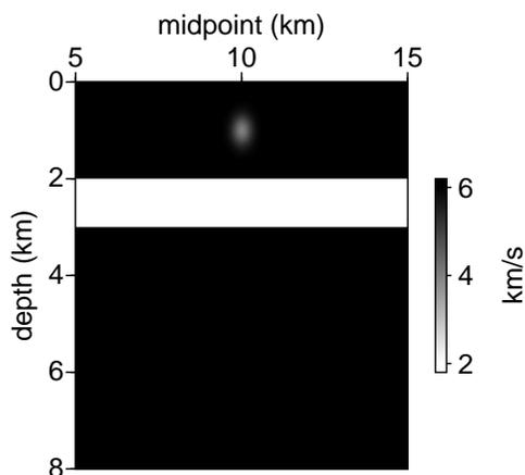
**Figure 7.** Velocity model, similar to the flat layered example discussed previously, with the addition of a low-velocity lens to demonstrate that the method works in laterally heterogeneous velocity models.
