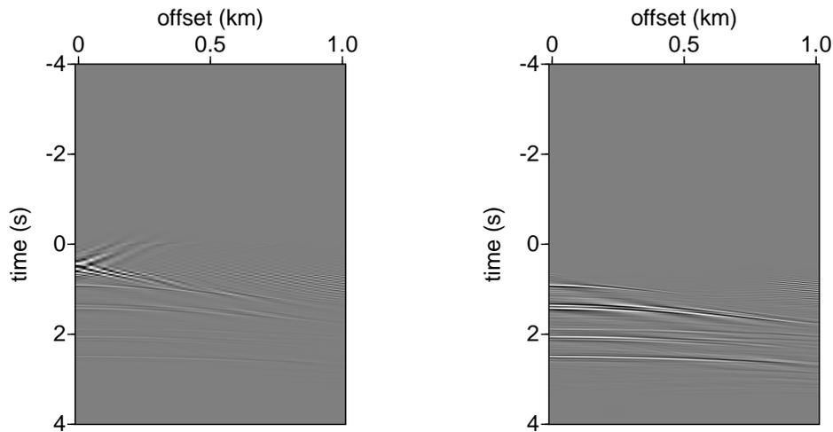
**Figure 18.** Data downward continued to a depth of 2.5 km. Left: before the removal of the part of the data at  $t \leq 0$ . Right: after the removal of the part of the data at  $t \leq 0$  using a  $\tau$ -p filter.
