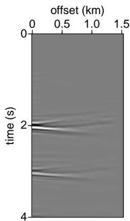
**Figure 10.** Top: Common midpoint gather at 9.8 km and 2 km depth. Note the disappearance of the multi-pathing as the data are now below the lens. Bottom: estimated multiples at this depth.
