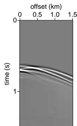
**Figure 9.** Common midpoint gather at 9.8 km, with only the offsets used to compute the images shown later. Note the triplications caused by the lens. Top: full gather. Bottom: zoom of the primary reflection from the top layer.
