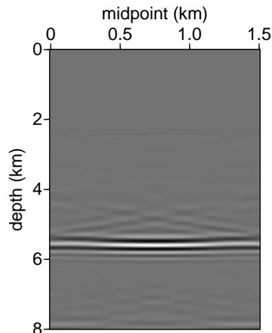
**Figure 6.** On the top is the image with an artifact from a first-order internal multiple at about 5.7 km depth. On the bottom is the estimated artifact.
