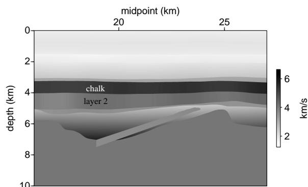
**Figure 17.** Velocity model for the North Sea example.
