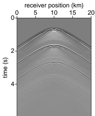
**Figure 8.** Shot record from  $s = 10$  km, directly above the lens. Note the caustic introduced by the lens around zero-offset. The ringing on the second primary (at about 2 s) and the multiple (at about 3 s) is most likely numerical dispersion from the modeling of the data.
