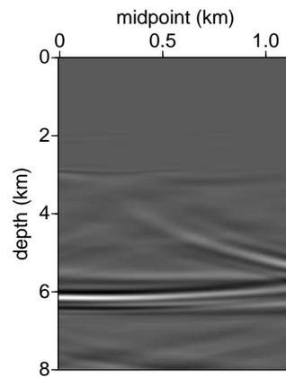
**Figure 14.** In these images, a second lens has been added beneath the layer to introduce a laterally varying velocity perturbation. Top: Image with artifacts from internal multiples. Bottom: Estimated artifacts from first-order internal multiples.
