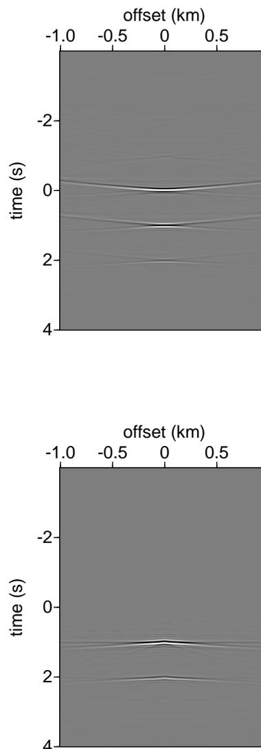
**Figure 4.** Data downward continued to the 1.5 km, the depth of the first reflector. Top: before the removal of the part of the data at  $t \leq 0$ . Bottom: after the removal of the part of the data at  $t \leq 0$ .
