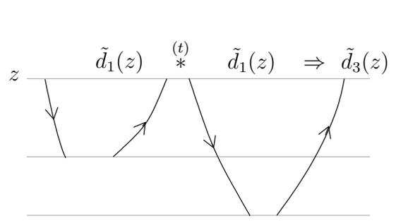
**Figure 2.** Illustration of equation 13, the estimation of the multiple at the depth  $z$ . The lines represent wavepaths rather than rays and do not connect as the imaging condition has not been applied.
