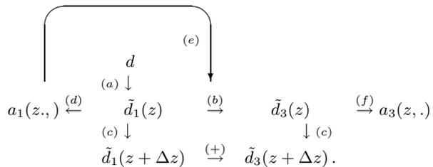
The algorithm can be divided into several steps. First, in (a), we downward continue the data to the depth  $z$ . Next we form an estimate,  $a(z, x)$ , of image from the data in (d). This estimate is used, in (b), to model the internal multiple downward continued to depth  $z$  via,
