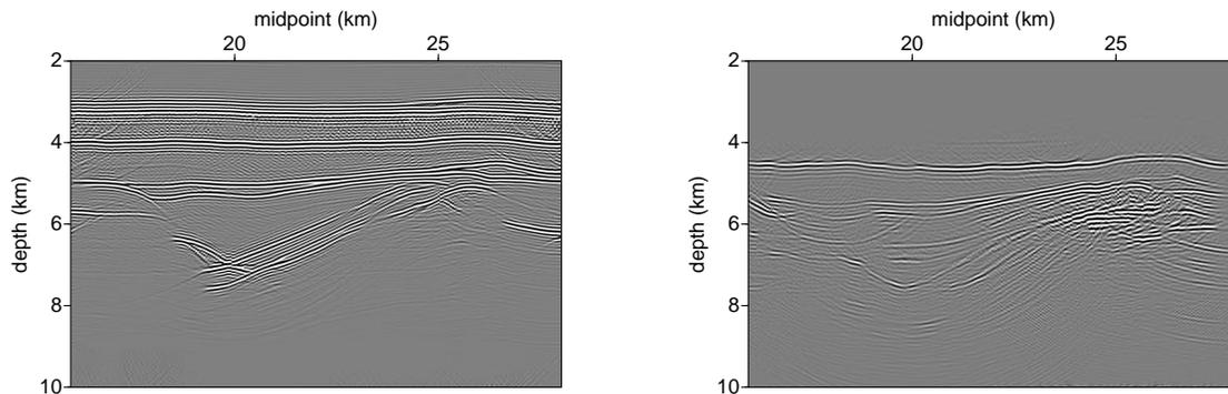
**Figure 19.** On the left is the image with an artifact from a first-order internal multiple at about 4.5 km depth. On the right is the estimated artifact.
