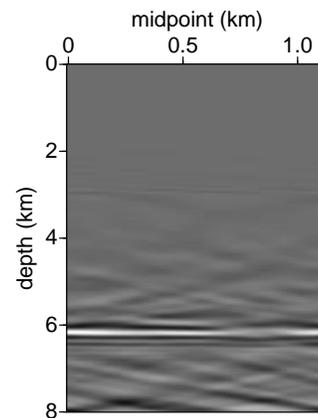
**Figure 11.** Top: Image with an artifact from the first-order internal multiple at approximately 6 km depth. Bottom: Estimated artifacts from first-order internal multiples.
