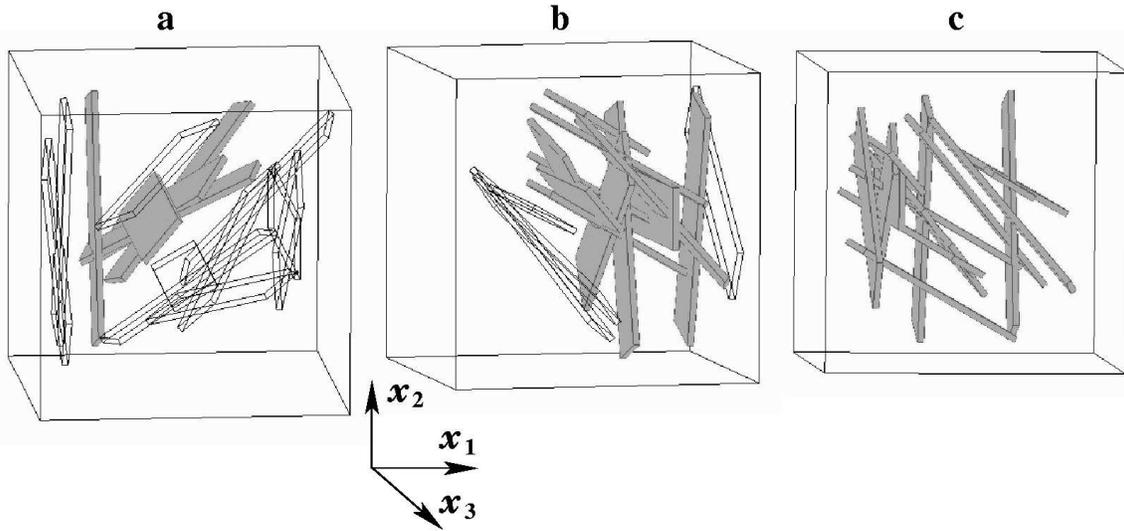
**Figure 5.** Models containing three sets of vertical rectangular cracks. Fractures that geometrically intersect their neighbors are shaded; isolated cracks are transparent. Cubes represent the rock volumes  $V$  indicating that the sizes of fractures and  $V$  are comparable.
