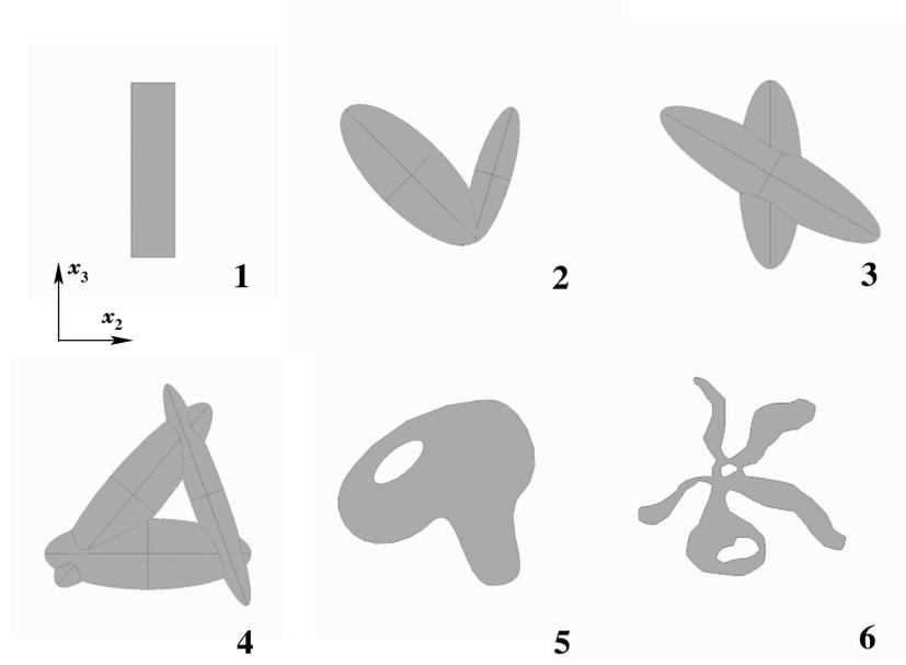
**Figure 1.** Fracture geometries used to study the influence of crack shape on the effective properties. All fractures are vertical and planar; their normals are directed along the  $x_1$ -axis. Geometries 4, 5, and 6 contain rock islands inside the cracks; these models represent partially closed fractures.
