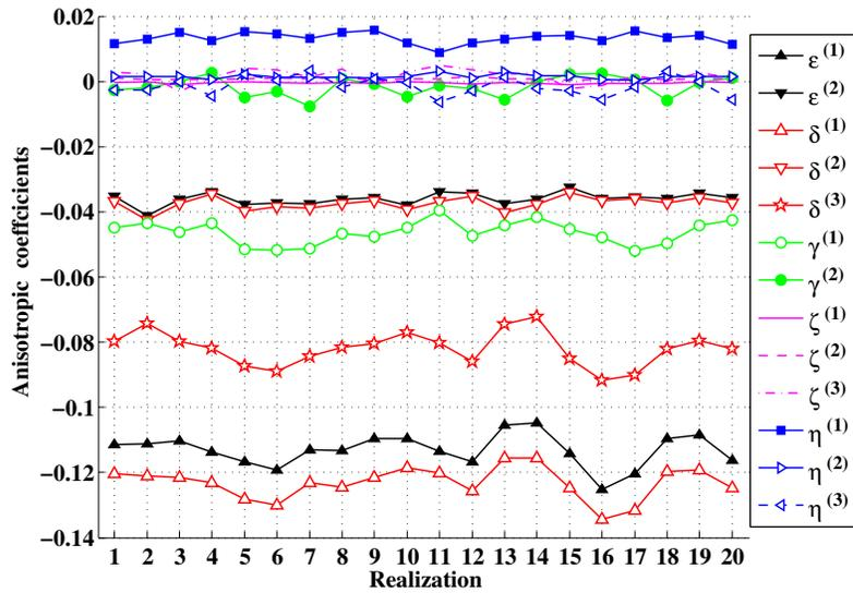
**Figure 6.** Effective anisotropic coefficients for models that contain three vertical sets of rectangular cracks.
