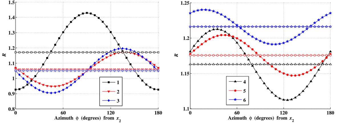
**Figure 2.**  $R(\phi)$  (solid symbols) and  $\langle R \rangle$  (open symbols) for fracture models 1 through 6 shown in Figure 1.
