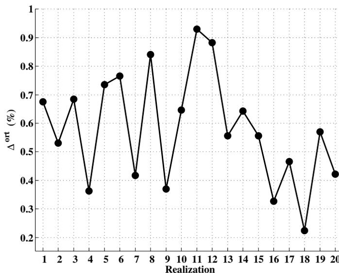
**Figure 7.** Relative deviations  $\Delta^{\text{ort}}$  of the effective stiffness tensors from orthotropy (equations 23, 24).
