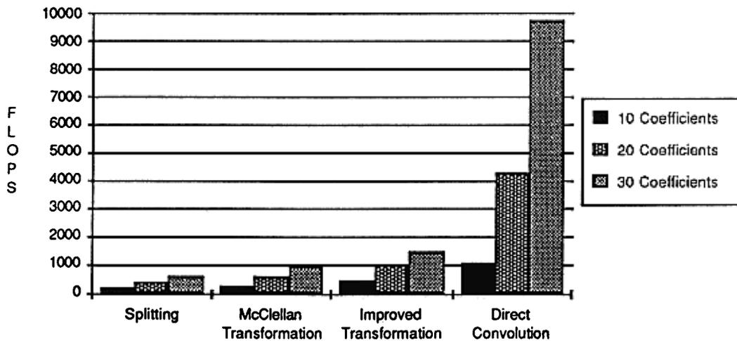
FIG. 12. Number of floating point operations (FLOPS) per output sample required by four different depth extrapolation methods. For each method, the number of FLOPS required is plotted for  $N_h = 10, 20,$  and  $30$  coefficients.
