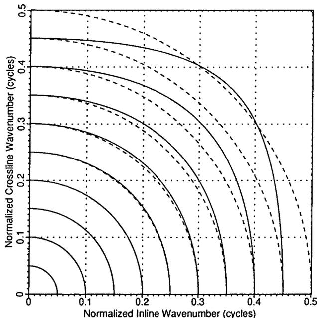
FIG. 5. Contours of constant amplitude and phase (constant  $k$ ) for two-dimensional filters designed and implemented via the improved McClellan transformation filter of Figure 4. Contours of ideal circularly symmetric filters are plotted with dashed lines. Compare with Figure 3. In this figure, normalized wavenumbers  $k_x$  and  $k_y$  are measured in cycles per spatial sampling interval. Thus,  $k = 0.25$  is one-half the Nyquist wavenumber.
