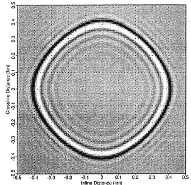
FIG. 10. Impulse response of 3-D migration via the original McClellan transformation, for the depth  $z = 250$  m. Compare with Figures 9 and 11.
