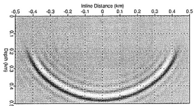
FIG. 6. Impulse response of 3-D migration via splitting, for the crossline coordinate  $y = 0$ . Compare with Figures 7 and 8.
