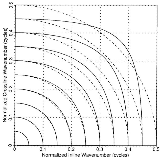
FIG. 3. Contours of constant amplitude and phase (constant  $k$ ) for two-dimensional filters designed and implemented via the original McClellan transformation of Figure 2. Contours of ideal circularly symmetric filters are plotted with dashed lines. Compare with Figure 5. In this figure, normalized wavenumbers  $k_x$  and  $k_y$  are measured in cycles per spatial sampling interval. Thus,  $k = 0.25$  is one-half the Nyquist wavenumber.
