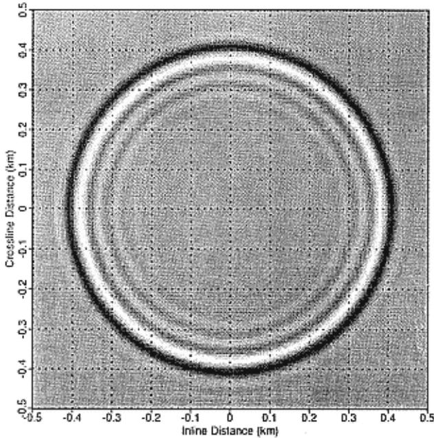
FIG. 11. Impulse response of 3-D migration via the improved McClellan transformation, for the depth  $z = 250$  m. Compare with Figures 9 and 10.
