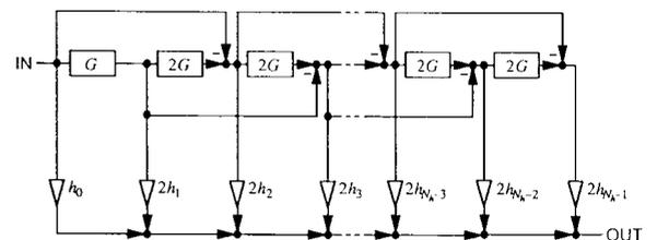
FIG. 1. Chebychev filter structure for convolution with the filter  $h_n$ . The upper part of this structure implements the Chebychev recursion for  $\cos(kn)$  in terms of  $G(k) = \cos k$ .
