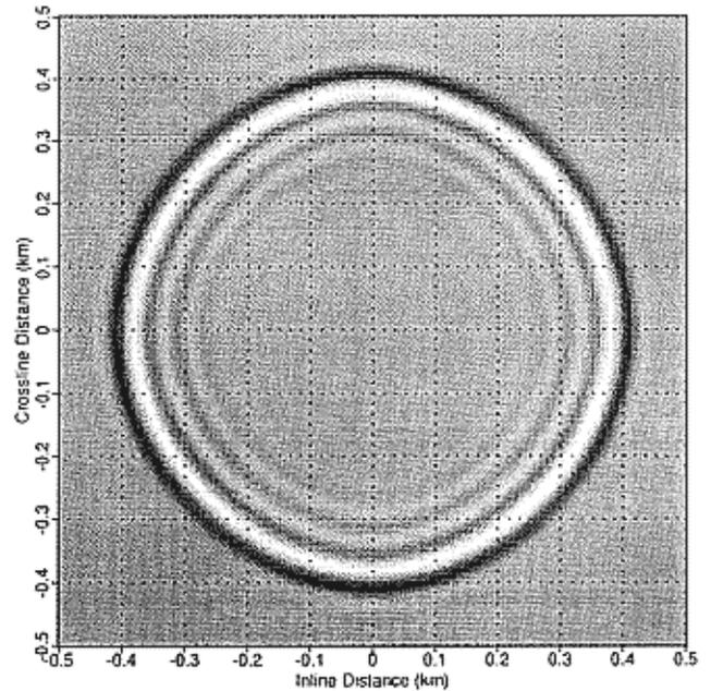
FIG. 9. Impulse response of 3-D migration via splitting, for the depth  $z = 250$  m. Compare with Figures 10 and 11.
