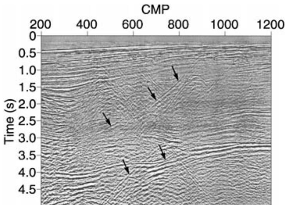
FIG. 5. Stacked section from offshore Africa, after applying NMO and isotropic homogeneous DMO. The arrows point to the sloping reflections used in the inversion for  $\eta(\tau)$ .
