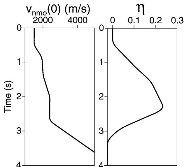
FIG. 6. Estimated interval values  $v_{\text{nmo}}$  and  $\eta$  as a function of vertical time.
