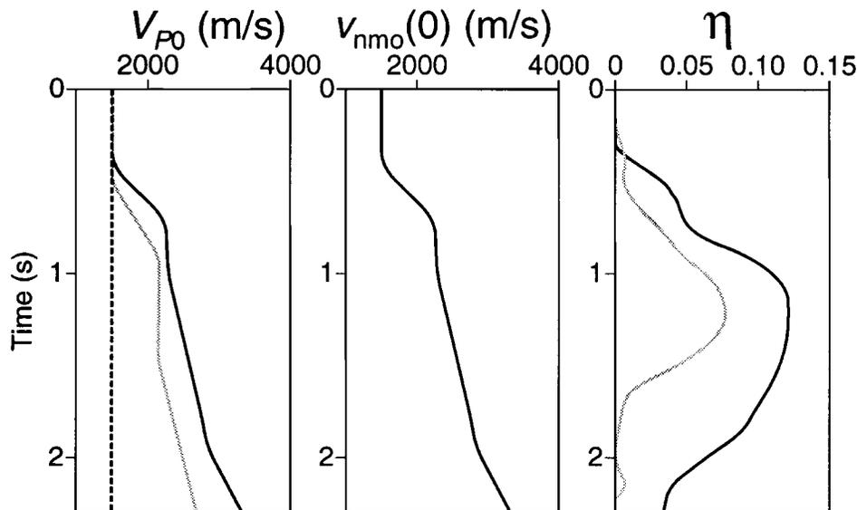
FIG. 1. Parameter variation as a function of vertical time. The parameters here correspond to the interval vertical velocity  $V_{P0}$ , the interval NMO velocity for horizontal reflectors  $v_{\text{nmo}}(0)$ , and the anisotropy parameter  $\eta$ . Different combinations of these parameters result in different models.
