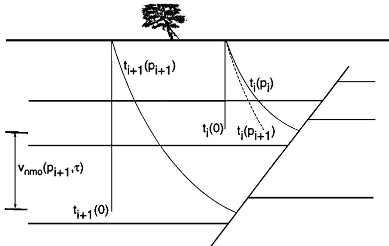
FIG. A-1. Depth model consisting of a fault and a number of horizontal layers. The rays drawn correspond to the measured stacking velocities ( $V_{\text{nmo}}[p_i, t_i(p_i)]$  and  $V_{\text{nmo}}[p_{i+1}, t_{i+1}(p_{i+1})]$ ) described in this Appendix. Such rays illustrate the relationship between the zero-offset time and the vertical time for reflections from the dipping fault.
