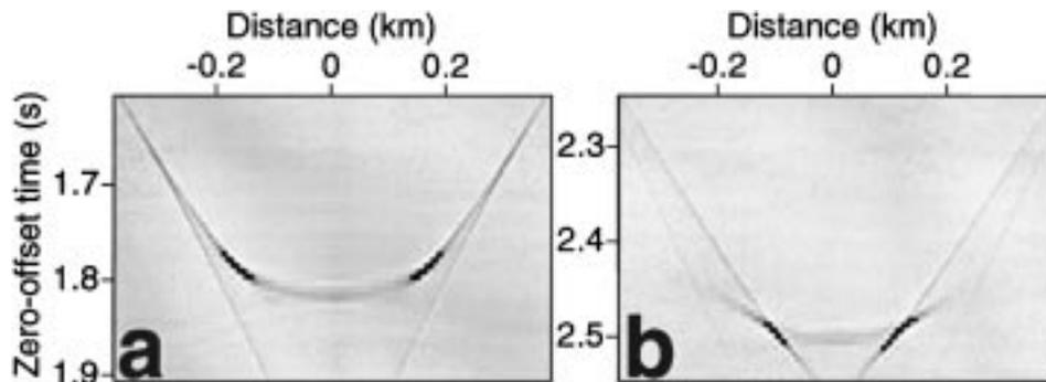
FIG. 8. VTI DMO impulse responses for the parameters in Figure 6. The offset is 1.5 km, and the apex is at (a) 1.8 s and (b) 2.5 s.
