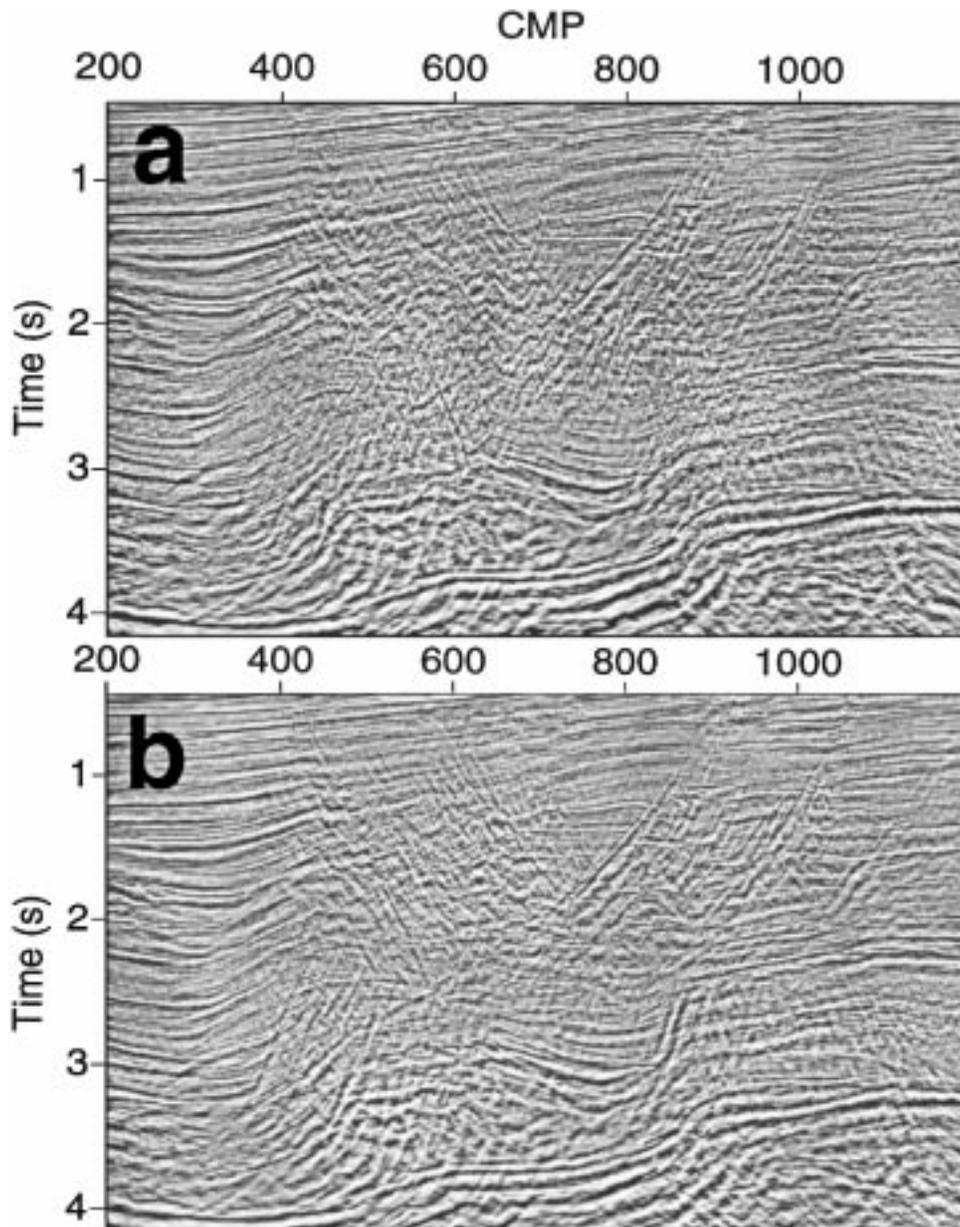
FIG. 10. Time-migrated section using (a) isotropic phase-shift migration of the data shown in Figure 5, and (b) anisotropic phase-shift migration of the data shown in Figure 7 using the parameters shown in Figure 6.
