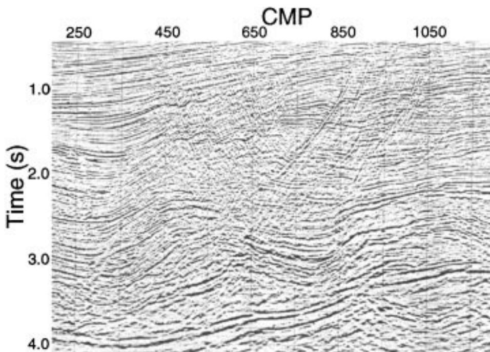
FIG. 4. Time-migrated section from offshore Africa based on conventional 3-D processing.
