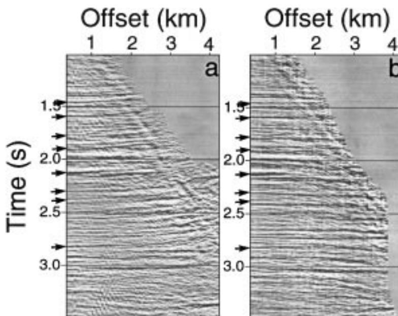
FIG. 9. CMP gathers for CMP location 700 after (a) homogeneous isotropic DMO, and (b)  $v(z)$  anisotropic DMO. The NMO correction, based on the velocities obtained from velocity analysis, is the same for both examples. The arrows point to some of the reflections from the dipping interfaces present in this gather.
