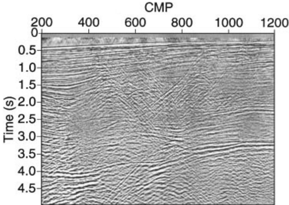
FIG. 7. Stacked section after  $v(z)$  anisotropic DMO using the parameters in Figure 6. The NMO correction is based on the velocities obtained from the conventional velocity analysis. Compare with Figure 5.
